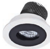
SD8223 Aluminum ● COB 7W color WH&BK/WH Cut-out: Φ80 Dimension: Φ95x87
