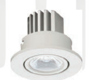
SD1202 Aluminum ● LED 1x3W BS/WH Cut-out: Φ55 Dimension: Φ67x51
